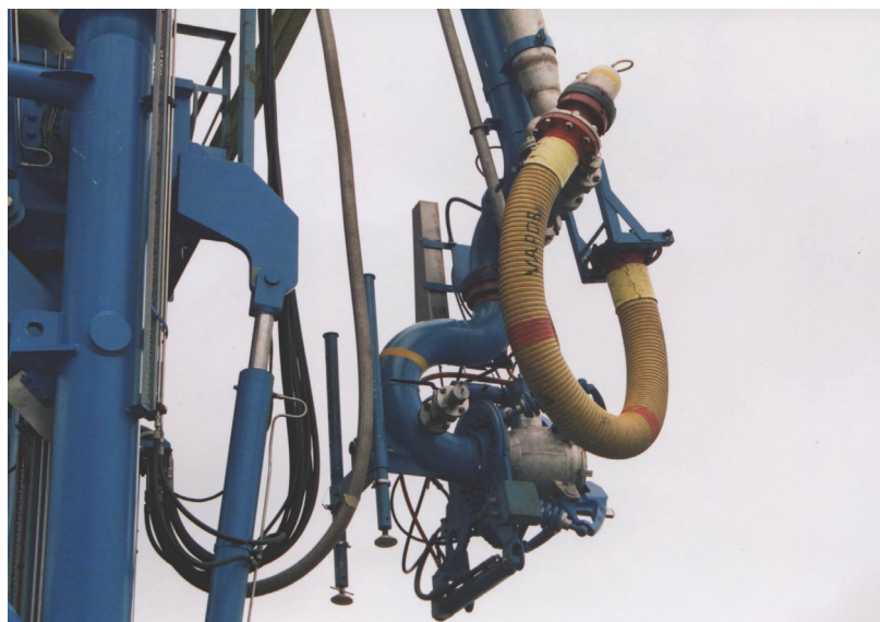
Figure 10 - close-up of vapour return facility
